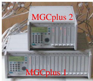
Fig. 6. MGCplus 1 and MGCplus 2 equipment
