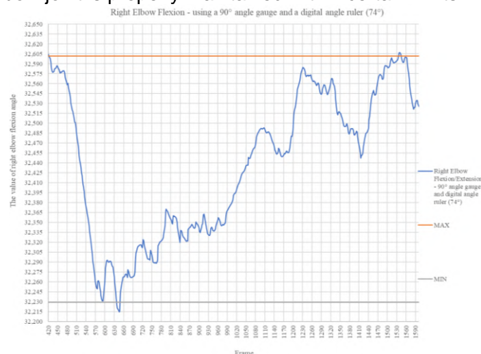
Fig. 6. The graphical representation of the amplitude of the variation of the flexion/extension angle at the level of the right elbow joint, blocked due to the positioning of the angle gauge inside it
