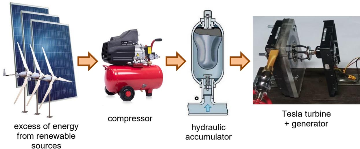
Fig. 2. Renewable energy storage scheme using a Tesla turbine
