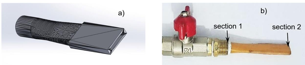
Fig. 3. Sketch (a) and view of the 3D-printed (b) jet nozzle
