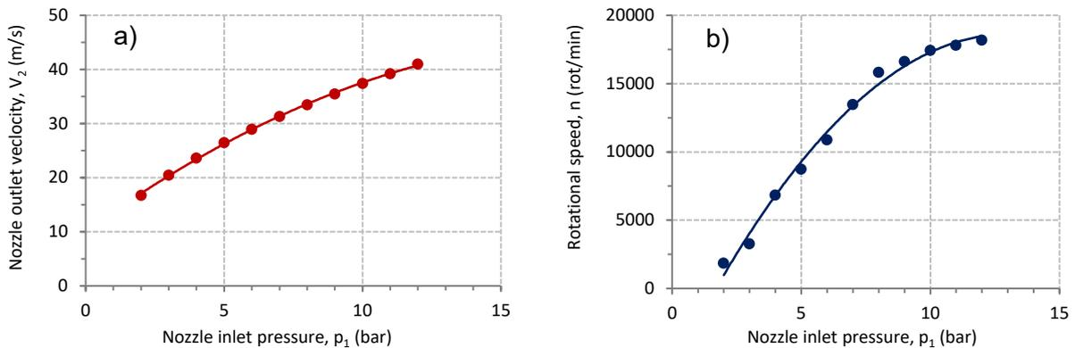
Fig. 7. Graphs with measurement results: nozzle velocity function of pressure (a) and turbine rotational speed function of pressure (b)
