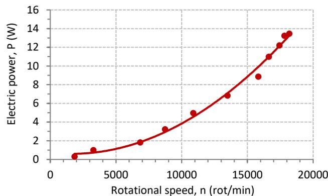
Fig. 1. Electric power produced by the turbine, function of rotational speed
