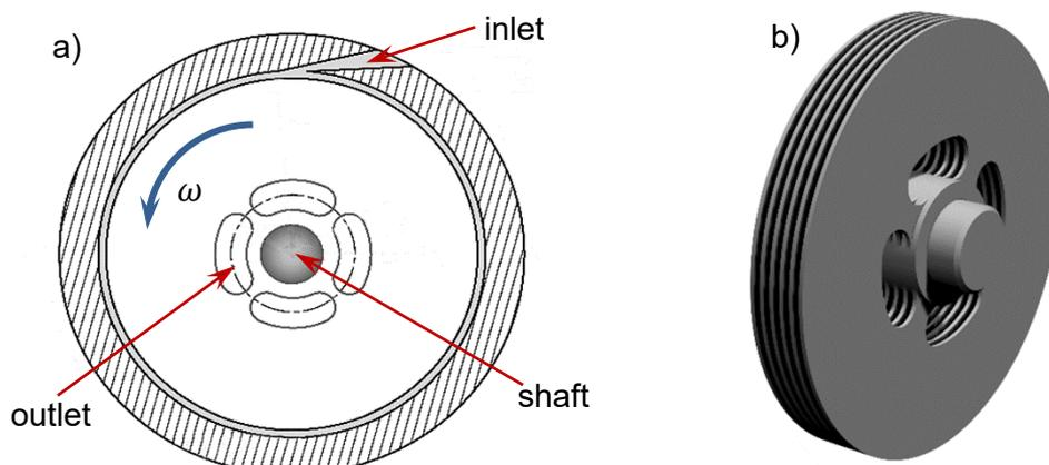
Fig. 1. Tesla turbine: schematic view (a) and 3D view of rotor (b) – adapted after [10]
