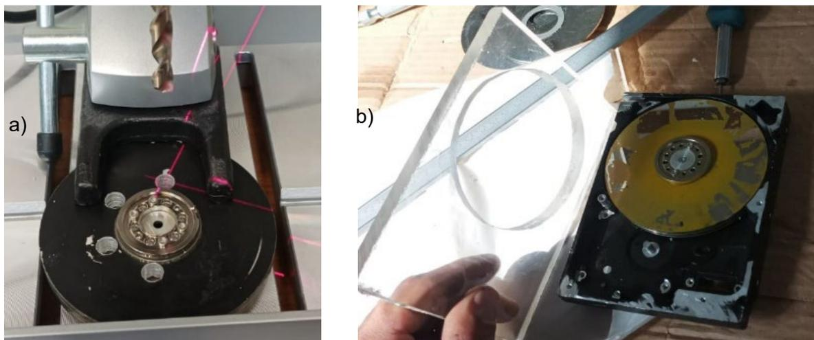
**Fig. 4.** Manufacturing the Tesla turbine for the experiments: turbine rotor (a) and case (b)
