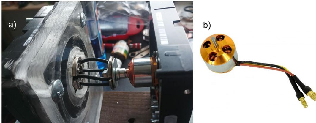
**Fig. 5.** The elastic coupling between turbine and generator shaft (a); the generator used for turning the mechanical power to electricity (b)
