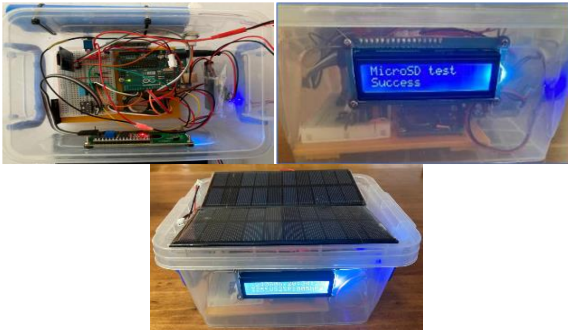
Fig. 1. Mini Weather Station - MSM 001 built on the STEM concept (top view, side view, view with solar panel)
