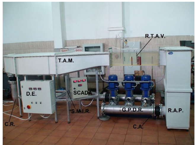
Fig. 3. The assembly of the main modules of the stand
