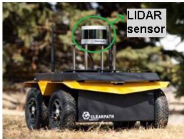
Fig. 3. Example of a LIDAR sensor mounted on a terrestrial robotic system [28]
