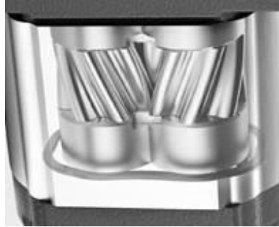
Fig. 1. External helical gear volumetric unit
