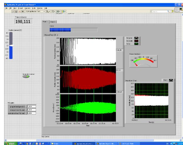
**Fig. 9.** Window 1 of the application for a stroke length of 30% of the total stroke, at an operating pressure of 8 bar, with a proportionality factor  $K_c = 1.000$  of the PID automatic controller, for the medium-pressure pneumatic actuator DNCKE-100-200-PPV-A
