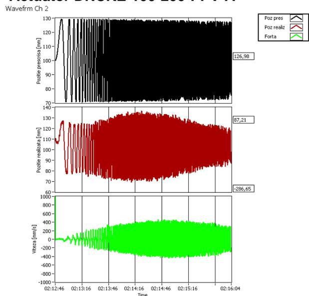
At the same values of the PID controller parameters, it is observed that amplitude attenuation begins within the first third of the frequency range (0...2 Hz).
