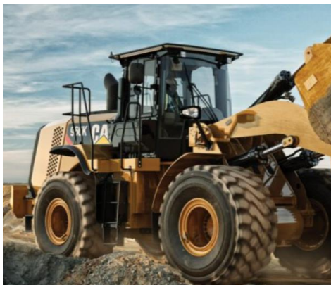
Fig. 5. Front loader with the 2 hydraulic cylinders driving the bucket
