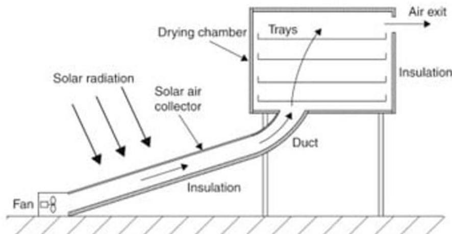
Fig. 2. Two-compartment dryer
