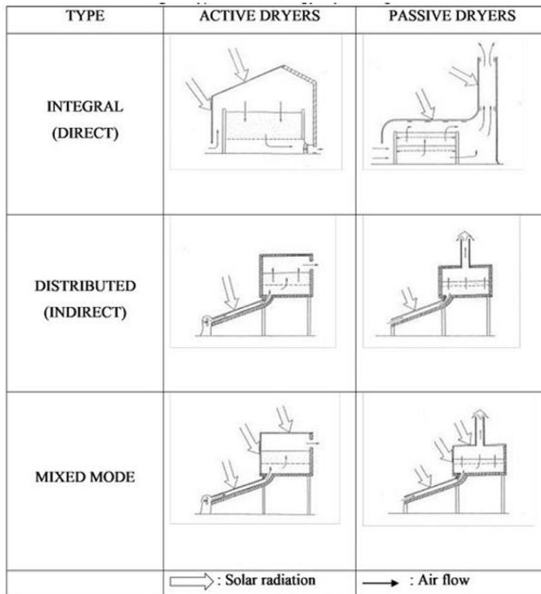
Fig. 1. Classification of solar-powered dryers
