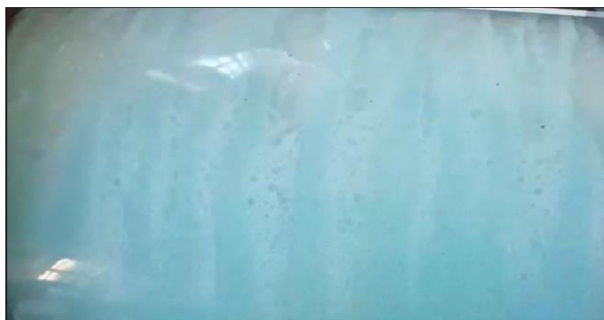
Fig. 4. Strings of vortices at speed n = 136 rot/min, Re = 37681 , Ta = 340438 , oil TR25.
