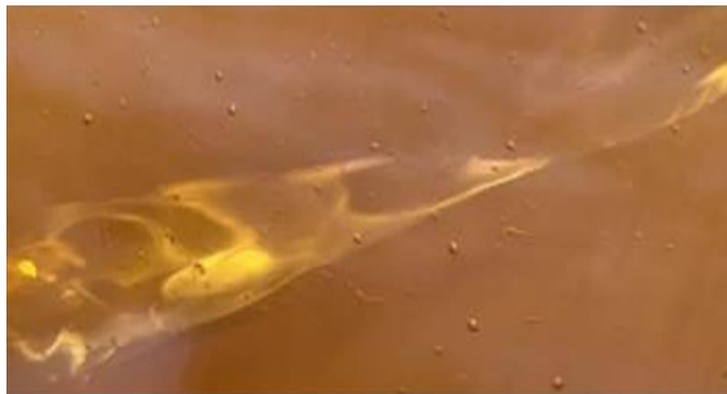
Fig. 6. The formation of Taylor vortices at speed n = 57 rot/min, Re = 892 , Ta = 191 , oil 80W90
