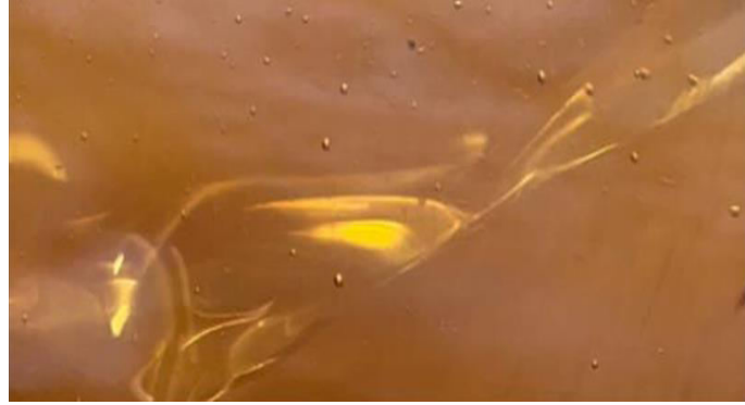
Fig. 7. The formation of Taylor vortices at speed n = 61 rot/ min, Re = 964 , Ta = 223 , oil 80W90.
