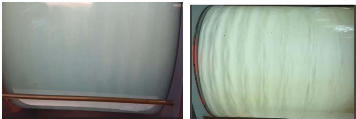
Fig. 3. Visualizations with the formation of Taylor vortex layers for TR25 and 80W90 oil respectively
