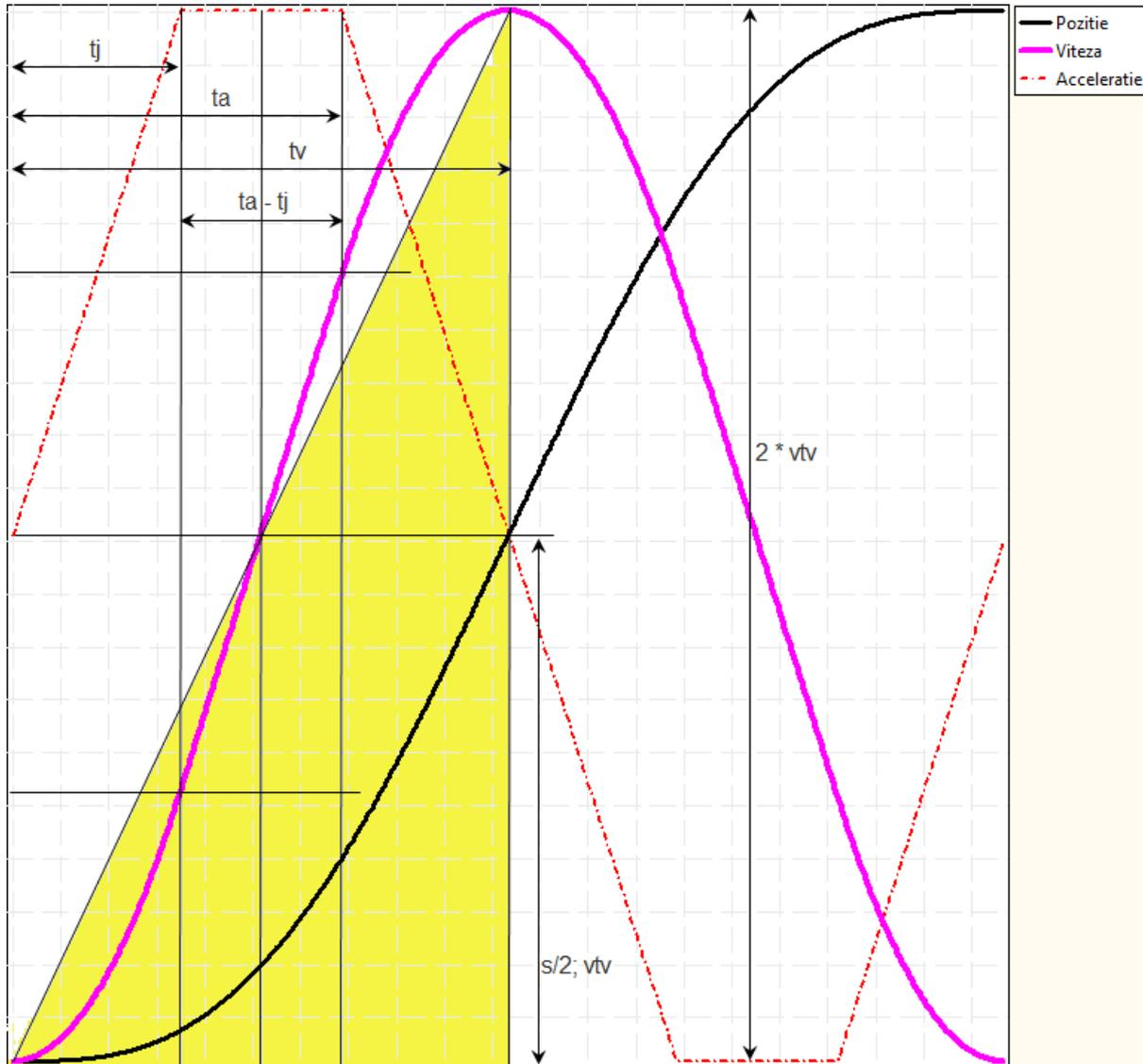
**Fig. 6.** Case D.2 - the value of the maximum acceleration is reached, the value of the maximum speed is not reached
