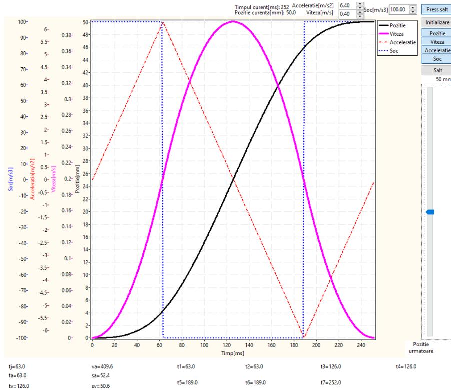
Fig. 15. Movement profiles B and C.2
