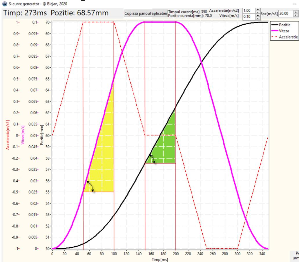
Fig. 3. Motion with acceleration and constant speed
