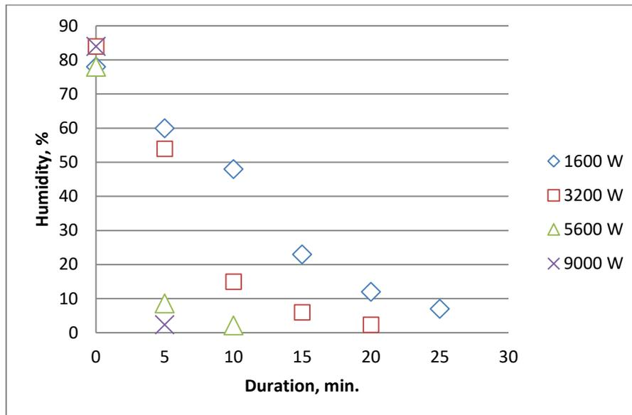
**Fig. 4.** Humidity profile depending on the duration for different microwave power levels
