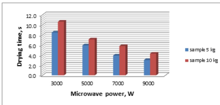
**Fig. 5.** Variation of drying time with microwave power
