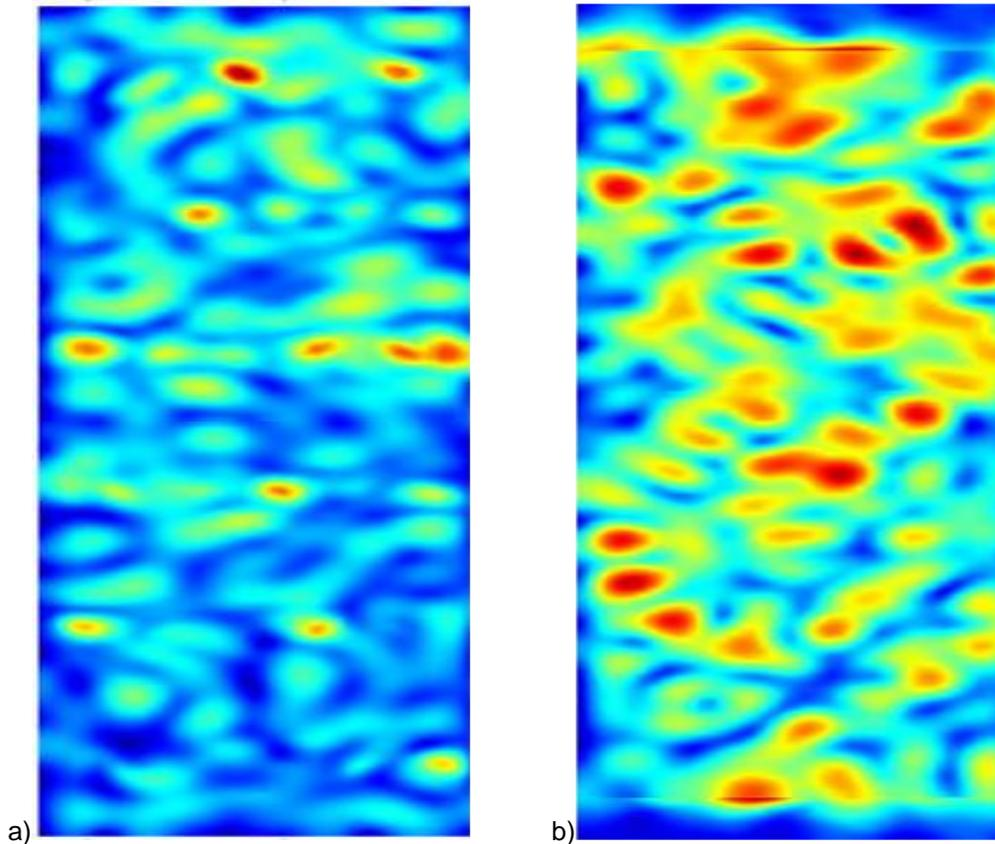
**Fig. 1.** Electric field distribution in the microwave - biomass arrangement plan: a) at 10 cm above b) at 1 cm above
