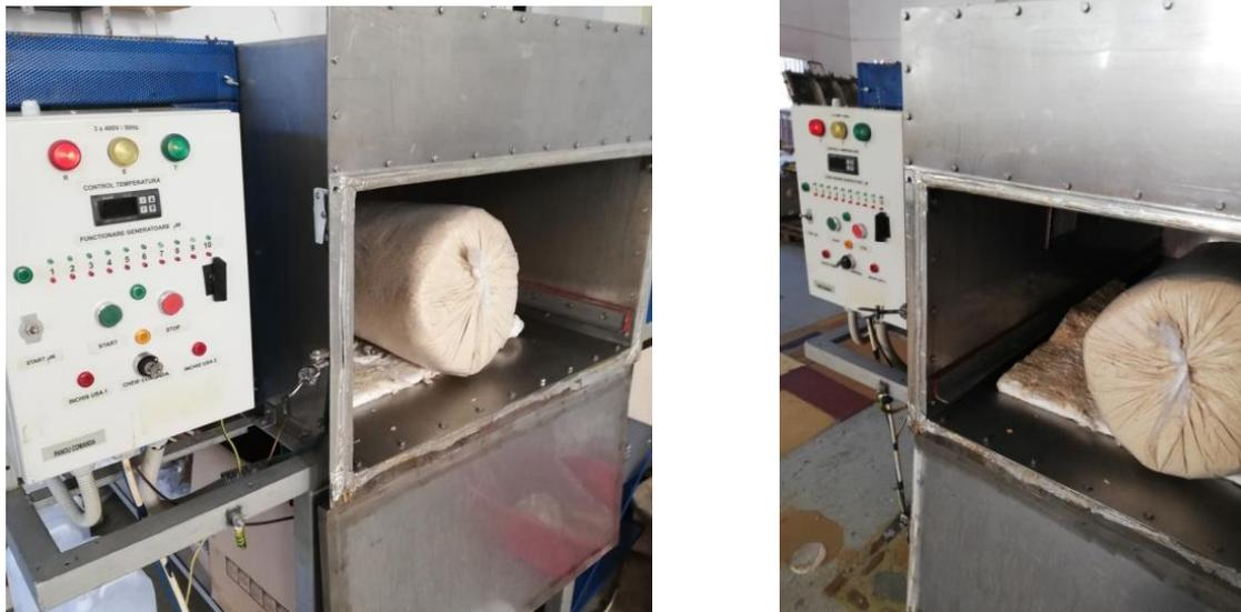
Fig. 3. Microwave-assisted drying equipment before testing, with biomass sample in cylindrical geometry
