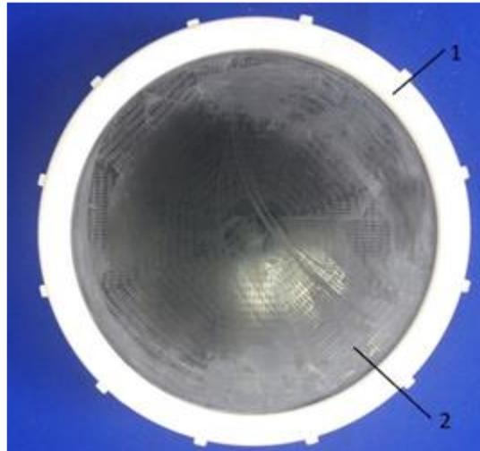
**Fig. 3.** Overview of the porous diffuser
