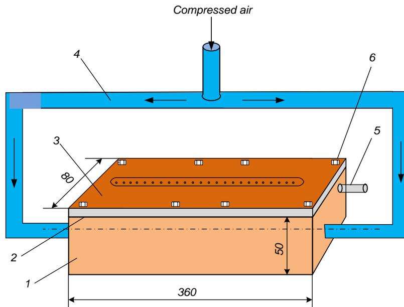
**Fig. 7.** Fine bubble generator with rectangular orifice plate
