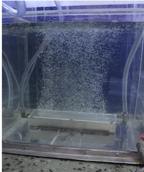
**Fig. 9.** Fine bubble generator in operation
